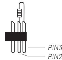
When using standard DMX512 control signal, the last device's output interface must be connected to a DMX plug. This plug is putting a 120 ohm resistance between "canon" plug's 2 pin and 3 pin. Showing as below pic. Sticking this plug into the last device's signal output interface, it will avoid the interference during the process of signal transmission.
