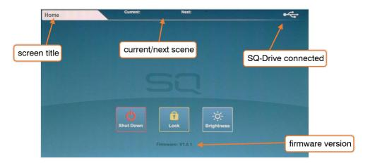
This is the first screen shown when powering on the SQ. It is also shown when no channels are selected, and no other screens are active.
