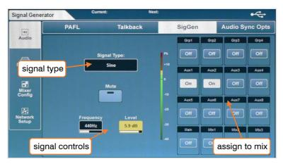
Touch the 'Signal Type' value to select a type of signal.
