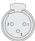
DMX-OUTPUT XLR mounting-sockets (rear view)
