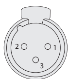
DMX-OUTPUT XLR mounting-sockets (rear view)
